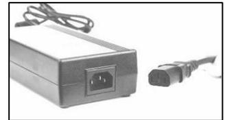
2. Connect the AC adapter to the power connector on the printer.
