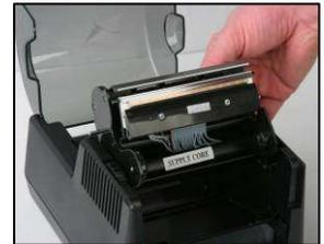
3. Place the left side of the ribbon supply core into the left supply core spindle.
