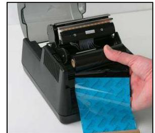
4. Gently pull the right spindle tab and place the right side of the ribbon core on the spindle.
