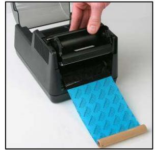
6. Align the notches on the left side of the ribbon take up core with the left spindle.
