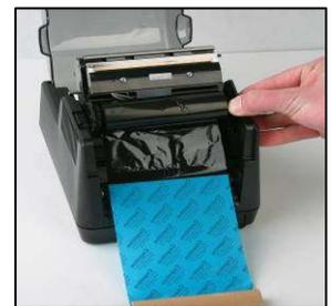
5. Lower the print head. Do not latch the printhead at this time.
